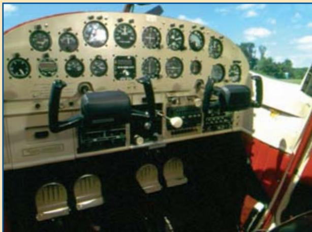
On the floor of the cockpit are pedals that operate the brakes and rudder. When the pilot pushes the right pedal, the rudder turns to the right. It will turn left when the left pedal is pushed.
